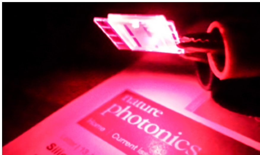
Operation of the ~740 nm OLED using Pt(II) complex 1. [Reproduced from Ref. 2]
